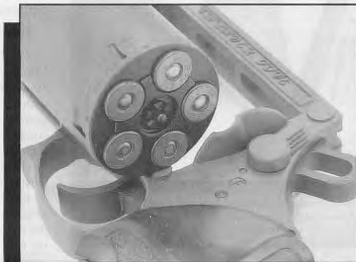
The Thunder Five's massive five-shot cylinder is not fluted and the chambers have no shoulder. Note half-inch-wide trigger, manual safety lever and hammer's distinctive oval-shaped cutout.
